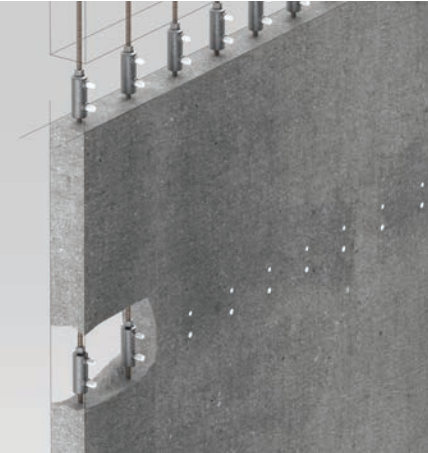
Shear Wall to Shear Wall
