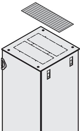
Flat top cover construction with cover plate
