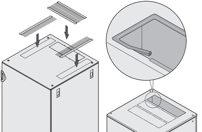
Flat top cover construction with brush strips
