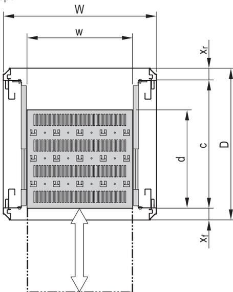
$c = \text{max. pitch of the } 19'' \text{ panel/slide mounts}$
