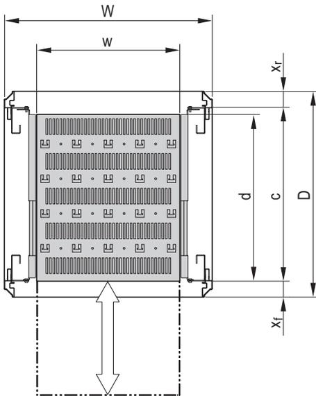
$c = \text{max. pitch for } 19'' \text{ panel/slide mounts}$
