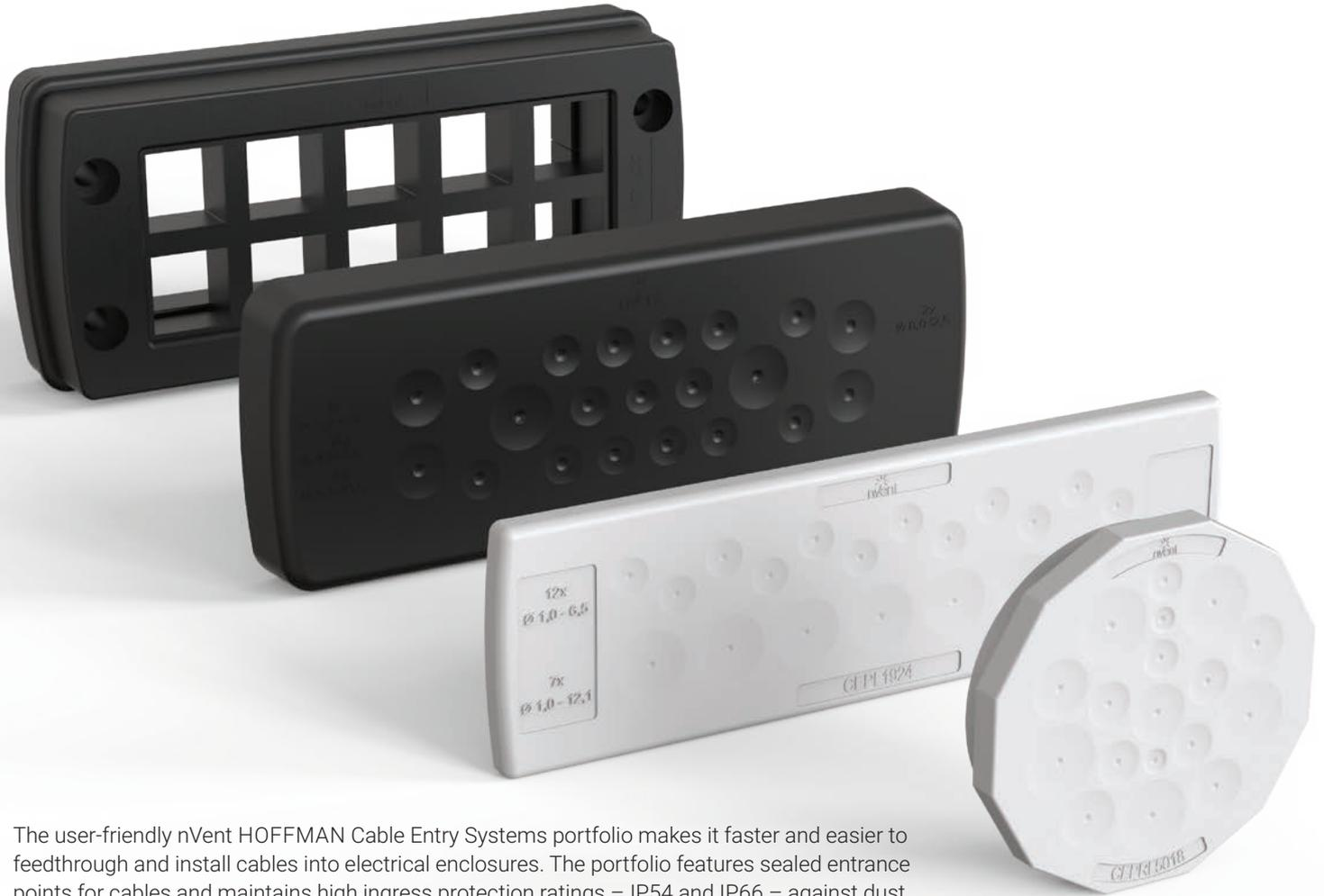
The user-friendly nVent HOFFMAN Cable Entry Systems portfolio makes it faster and easier to feedthrough and install cables into electrical enclosures. The portfolio features sealed entrance points for cables and maintains high ingress protection ratings – IP54 and IP66 – against dust, water and vibration.
