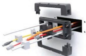
Fast, safe and versatile modular cable entry system provides secure seals and strain relief for pre-assembled and unassembled cables with or without connectors. Made of a sturdy, glass-fiber reinforced plastic. The system comes prepared with inlays to fit small grommets.
