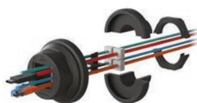
Quick and easy to assemble, consisting of CCFR Frame, CCFRM Adaptor and CCFRM counter Nut, CCFR secures seals and strain relief for pre-assembled and non-assembled cables with or without connectors. Managing everything from the outside of the enclosure and without the need to disassemble and reconnect connectors on cables, the manufacturer's warranty is not voided. The frames, inlays and grommets can be combined in multiple ways, ensuring many versatile configuration options.
